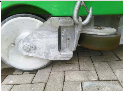
Cracked Caster on Vehicle
