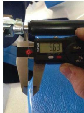
Lap bar closed position – creep measurement
