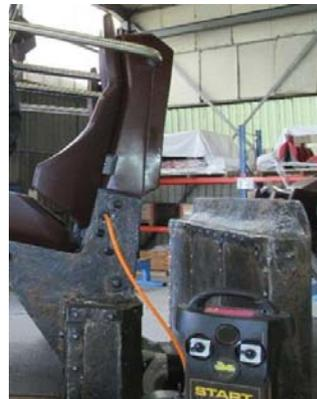
Test Box Connection on Coaster Vehicle
